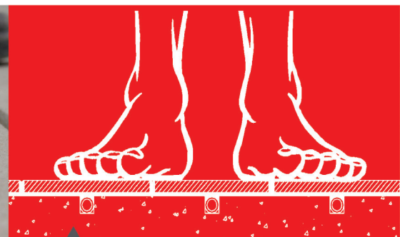
Heating pipes are installed directly under the surface of the floor, for quick heating and precision room temperature control.
